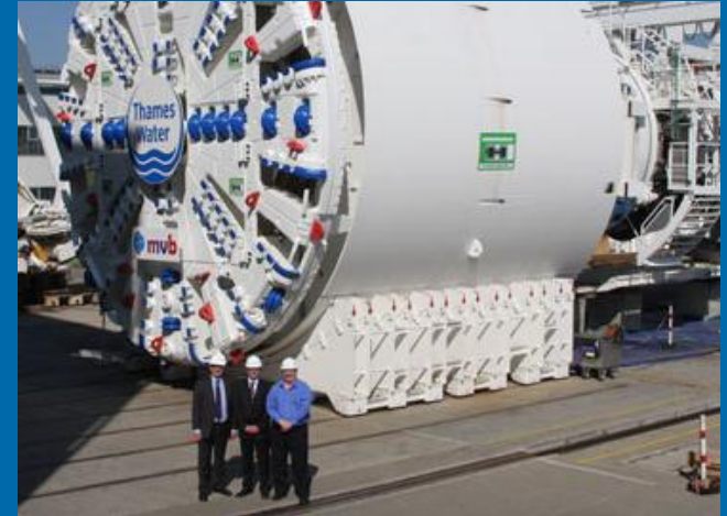
“Busy Lizzie” – the 7m diameter tunnelling machine
